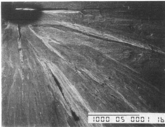
Fig. 6. Fracture surface of calcium phosphate glass crystallized at 570°C.
